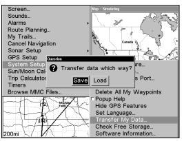
The Transfer My Data submenu asks if you want to save data to the MMC or load data from the MMC into the unit's memory.
